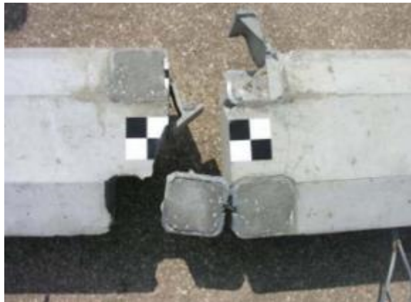
Figure 2.17 Failed MWRSF I-Shaped rail connection ( MWRSF, 2012 )
