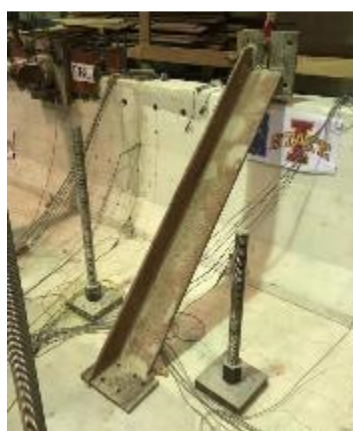
Figure 5.24 Beam used to brace PBU with respect to the deck during Test 4
