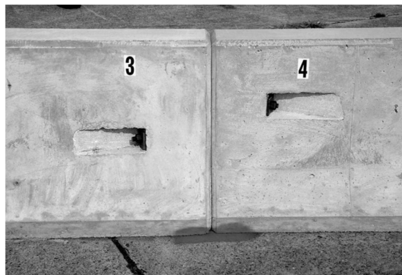
Figure 2.11 X-Bolt test specimen ( TTI, 2005 )
