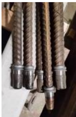
Figure 4.13 Threaded end of inclined reinforcement
