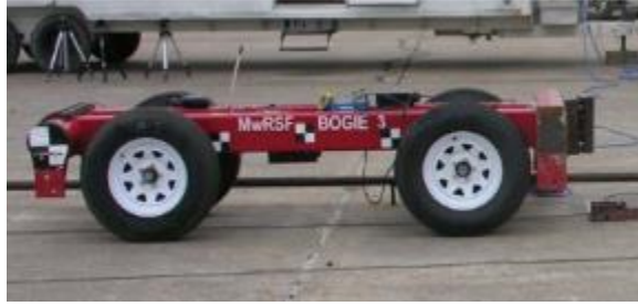
Figure 2.14 Impact bogie vehicle ( MWRSF, 2012 )
