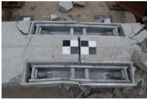
Figure 2.25 Side bolt and shear tube connection after testing (MWRSF, 2012)
