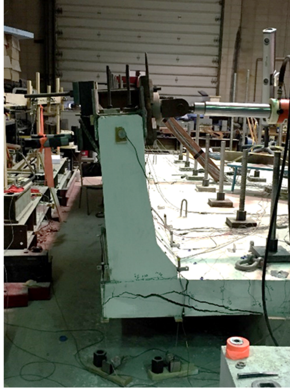
Figure 5.33 Final barrier deflection and cracking in bridge deck during push direction loading in Test 5
