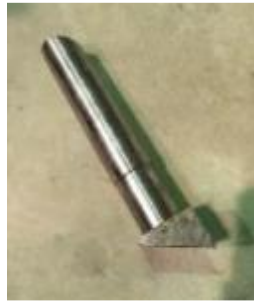
Figure 4.6 Inclined bar connection in deck
