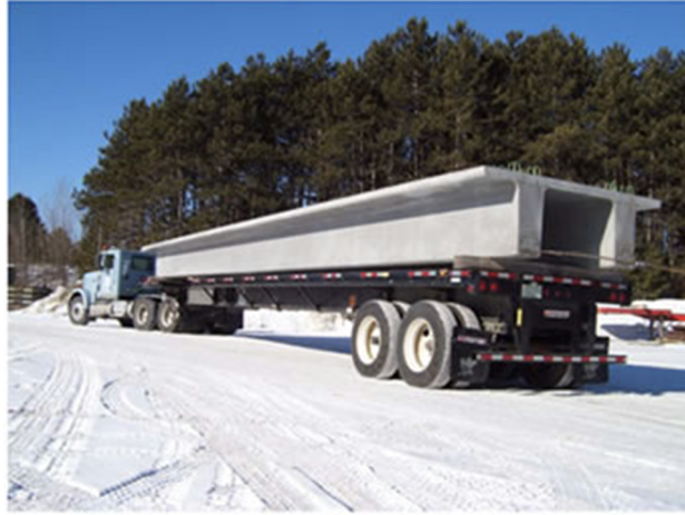
Figure 1.2 Prefabricated bridge element ( Courtesy of FHWA )
